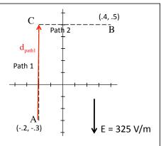
As the voltage doesn't change along Path 2, the voltage difference between A and B must be the same as the voltage difference between A and C, or 260 volts.
