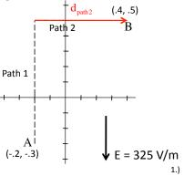
For Path 1: Defining *d* to start at Point A and terminate at Point C, notice that the angle between *E* and *d* is 180 degrees, relative to one another. That means that
